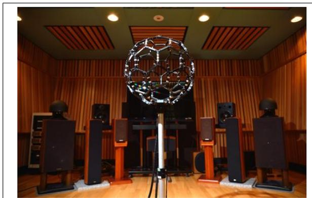
Figure 4. BoSC microphone array.
