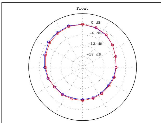
Figure 13. Relative SPLs of BoSC microphone array (Original speaker direction:  $90^\circ$ , blue: original, red: reproduced)
