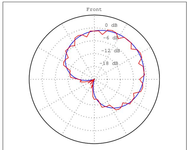
Figure 5. Simulation of sound directivity reproduction (Original source direction:  $45^\circ$ , measurement radius: 2 m, original: blue line, reproduced: red line)
