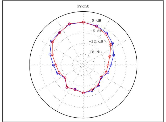
Figure 11. Relative SPLs of the BoSC microphone array (Original speaker direction: 0°, blue: original, red: reproduced)
