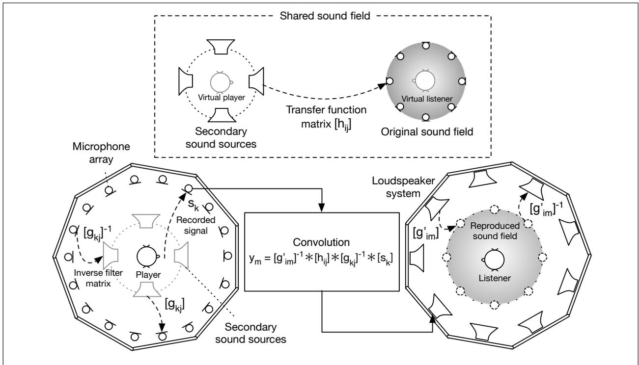
Figure 2. Sound directivity reproduction system for use in telecommunication
