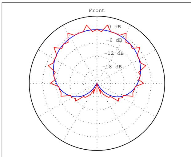
Figure 7. Simulation of sound directivity reproduction (Original source direction:  $0^\circ$ , measurement radius: 3.0 m, original: blue line, reproduced: red line)
