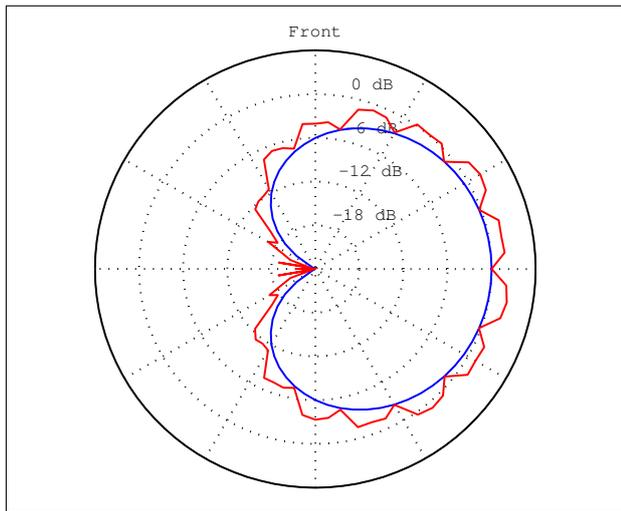
Figure 6. Simulation of sound directivity reproduction (Original source direction:  $90^\circ$ , measurement radius: 2 m, original: blue line, reproduced: red line)
