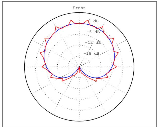
Figure 8. Simulation of sound directivity reproduction (Original source direction:  $0^\circ$ , measurement radius: 0.5 m, original: blue line, reproduced: red line)
