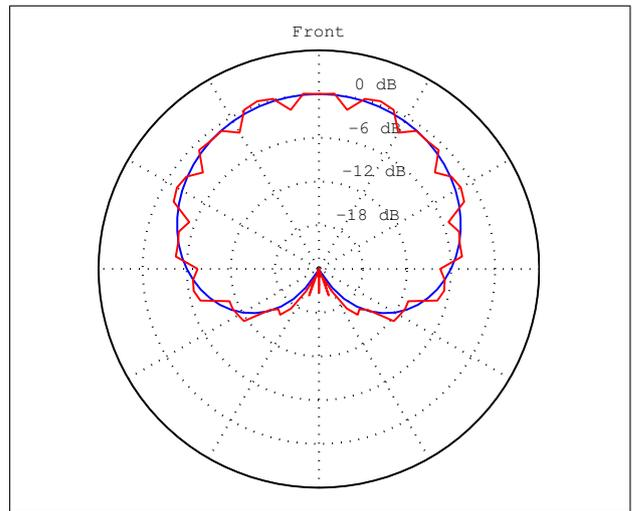
Figure 4. Simulation of sound directivity reproduction (Original source direction:  $0^\circ$ , measurement radius: 2.0 m, original: blue line, reproduced: red line)
