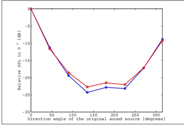
Figure 10. Relative SPLs at the front of the BoSC microphone array (Blue: original, red: reproduced)
