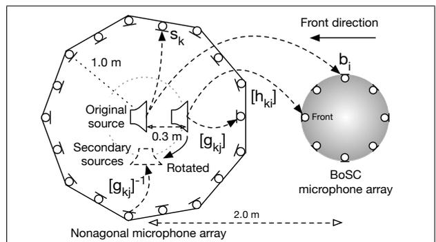
Figure 9. Conditions for experiments in an anechoic chamber
