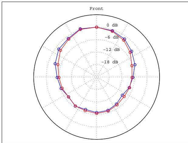
Figure 12. Relative SPLs of BoSC microphone array (Original speaker direction:  $45^\circ$ , blue: original, red: reproduced)
