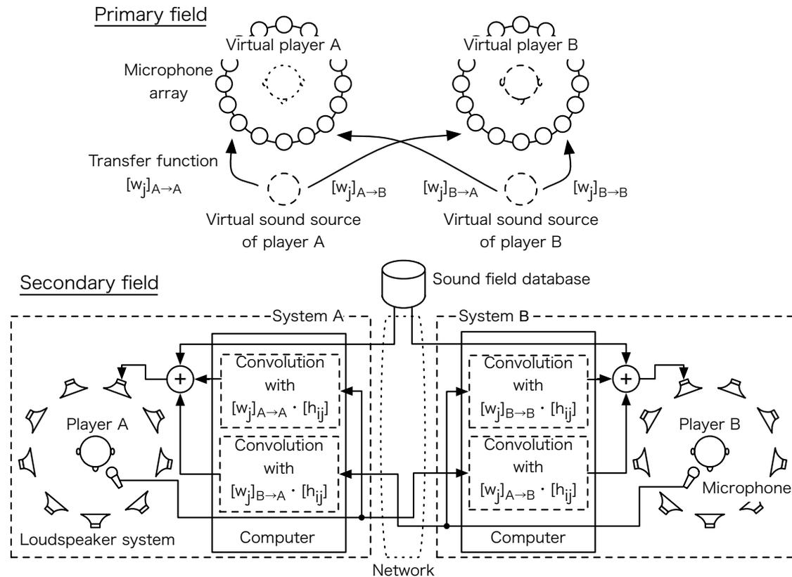
FIGURE 5: Signal flow of the sound field sharing system using sound casks.
