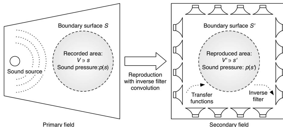
**FIGURE 1:** Concept of sound field reproduction based on the boundary surface control principle.
