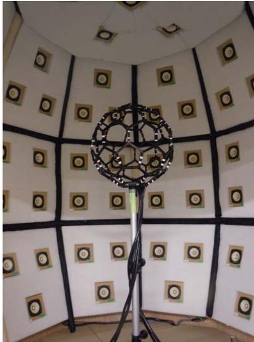
**FIGURE 4:** Microphone array for BoSC in a sound cask to record transfer functions.
