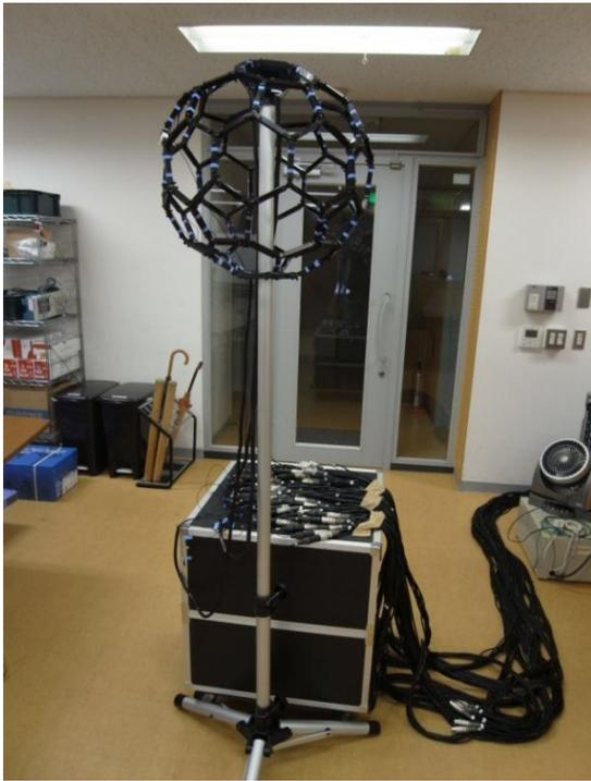
Fig. 1. C80 fullerene structure microphone array to record a 3D sound field with 80 nodes having intervals of around 8 cm. 70 omni-directional microphones are installed on each node position except 10 nodes of downside part.
