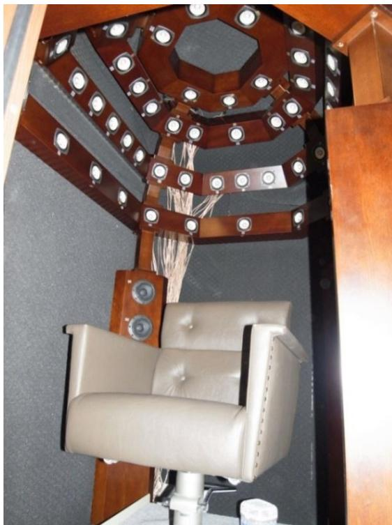
Fig. 2. Loudspeaker system to reconstruct a 3D sound field recorded by a C80 fullerene-structured microphone array that consists of a dome structure and a support pillar. The dome structure part has four mounting racks and six full-range units, and 16, 24 and 16 units are installed on them, respectively.
