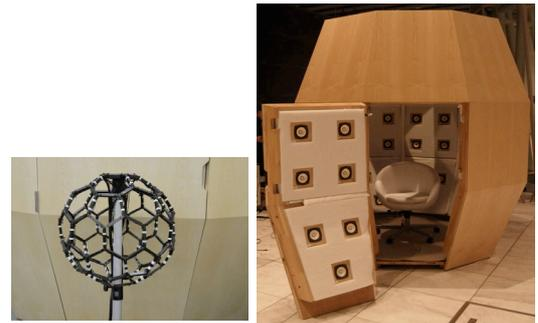
Figure 1. the BoSC microphone system (left panel) and the Sound Cask (right panel)
