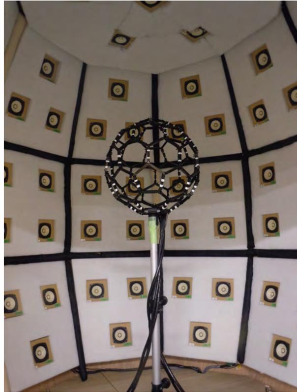
**Fig. 4:** BoSC microphone array placed in the sound cask for measuring transfer functions to design the inverse system.
