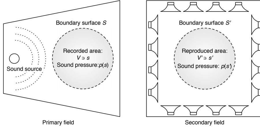
**Fig. 1:** Concept of the boundary surface control principle.
