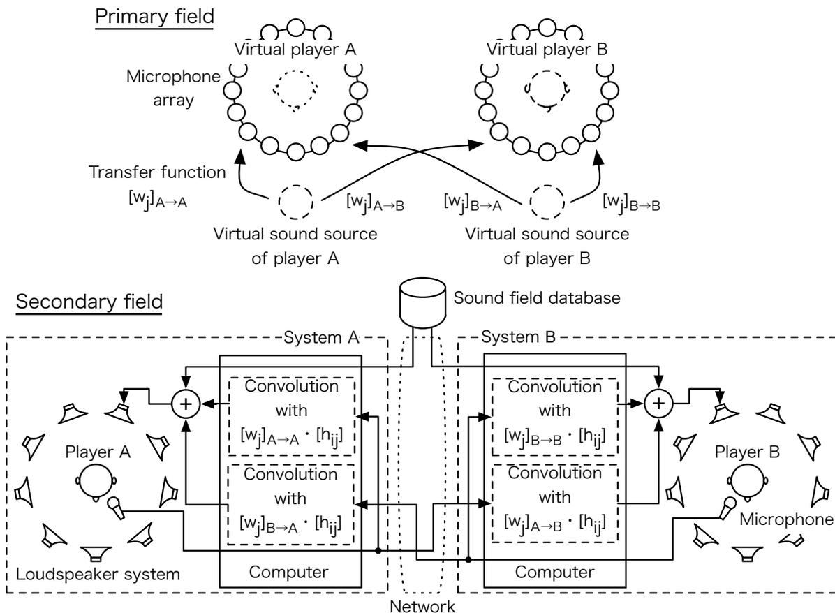
**Fig. 6:** Sound signal flow of the sound field sharing system with sound cask.
