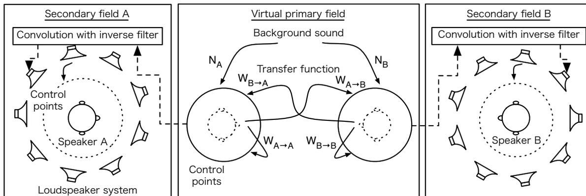
Fig. 2: Concept of the sound field sharing system.
